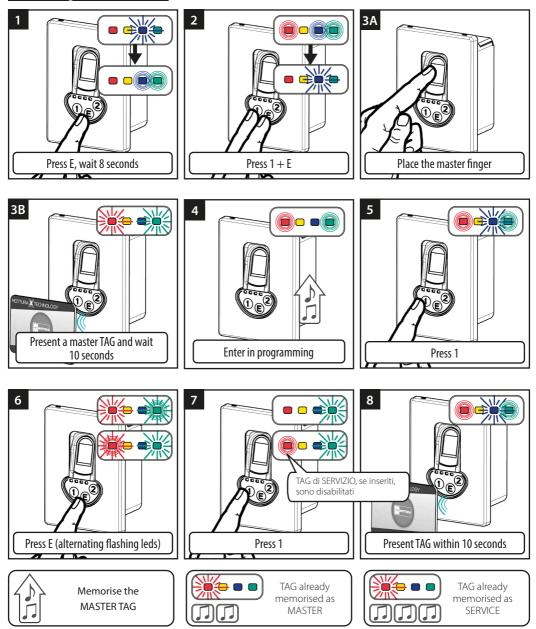
The system returns to point 7 To end press "E" or wait 20 seconds (exit time - timeout)
