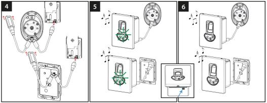
Disconnect the key from the cable and Press the programming button on the Press the button again until hearing a beep connect the cable to the accessory on the accessory within the limit of the required in the accessory that indicates the beginning USB-C connector. GREEN led flashes.
