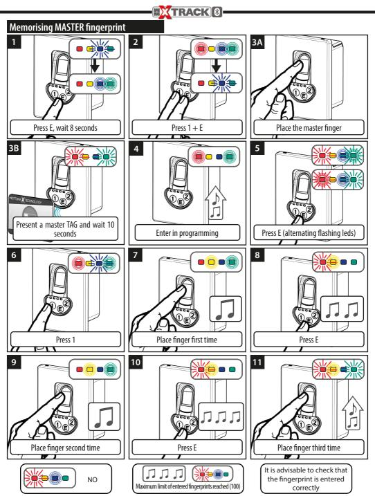
The system returns to point 3. To memorise another fingerprint (max 100) repeat the operations from point 4. To end press E or wait 20 seconds (exit time - timeout).
