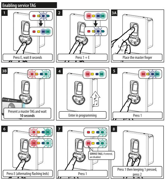
The system returns to point 7 To end press "E" or wait 20 seconds. (exit time - timeout)
