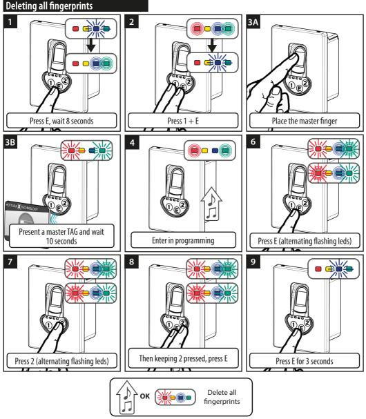
The system returns to point 3. To end press E or wait 20 seconds (exit time - timeout).
